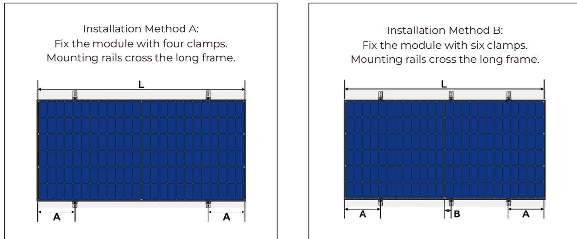
The Maximum Test Load of Mono-Facial Module Installation
